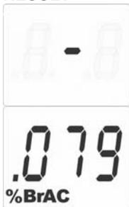
As soon as a successful breath sample has been captured, the analyzing signal “\_ \_ \_”, “\_ - \_”, “\_ \_ -” is scrolled across the display. At the end of the analysis a result will be displayed.
