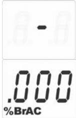
*Depending upon the version of the Alco-Sensor FST, the result may be displayed in two digits, three digits or 0 (Zero), PAS (Pass), CAU (Caution), FAil (Fail), and the unit of measure may or may not be displayed.*
