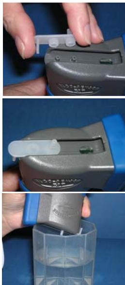
To test a beverage for the presence of alcohol, attach the 'mouthpiece drink sniffer' and put the instrument in the Passive Mode with "PAS" flashing.
