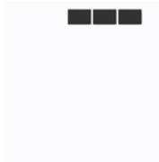
The FST is designed to perform repeat Quick Screen Tests while in the Road Block Testing Mode. After the result is displayed the instrument will go into a low power mode for two minutes. This mode is indicated by a dash slowly moving across the top of the display. Once in the low power mode there are three possible events that can change the instrument’s mode of operation:
