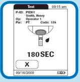
The test strip symbol appears after a few seconds with a flashing drop of blood. You have 180 seconds to apply the sample.
