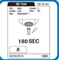
The dropper icon flashes to indicate that the meter is ready to perform the test.
