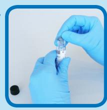
Carefully remove the screw cap and rubber stopper from the quality control bottle and make sure that none of the dried powder is removed with the rubber stopper. **3.**
