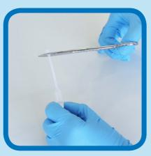
Holding the dropper at the bottom of the stem use scissors to cut off the tip of the dropper at the <u>upper end of</u> <u>the stem.</u> Do not squeeze the bulb of the dropper. 4.
