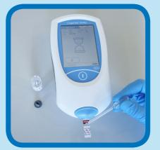
Mix the control again by gently swirling. Draw the solution into the dropper and apply one hanging drop to the clear target area and the meter will beep when the control sample is detected and the INR measurement begins.
