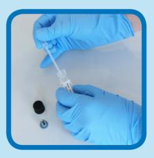
Insert the dropper tip first, into the control solution bottle. Gently squeeze the bulb to dispense the entire contents of the dropper onto the dried powder. Do not touch the dried material and the dropper. **5.**
