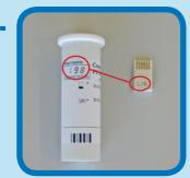
Make sure you have the code chip ready to insert if you are opening a new box of strips. The code chip needs to be inserted into the meter everytime you use a new lot of strips.
