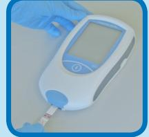
Slide the test strip into the test strip guide in the direction of the arrows until it stops.
