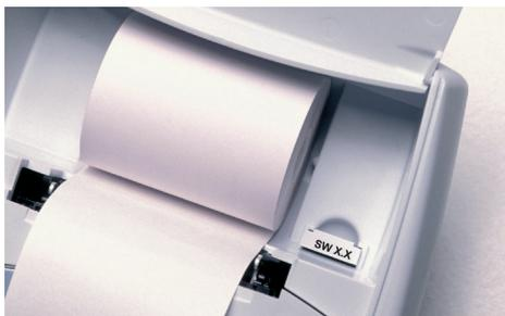
**1** Open printer cover by pressing area directly below and to the right of the printer paper slot. Remove the old paper roll.
